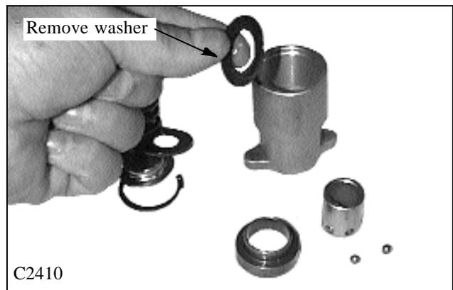
37 Clean all parts with solvent. Lubricate all parts with Castrol Spheerol grease or equivalent.
