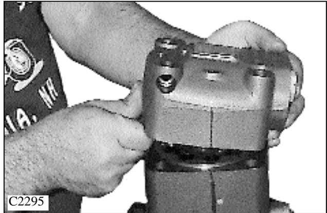
10 Remove the channel plate. (fig. C2296)
