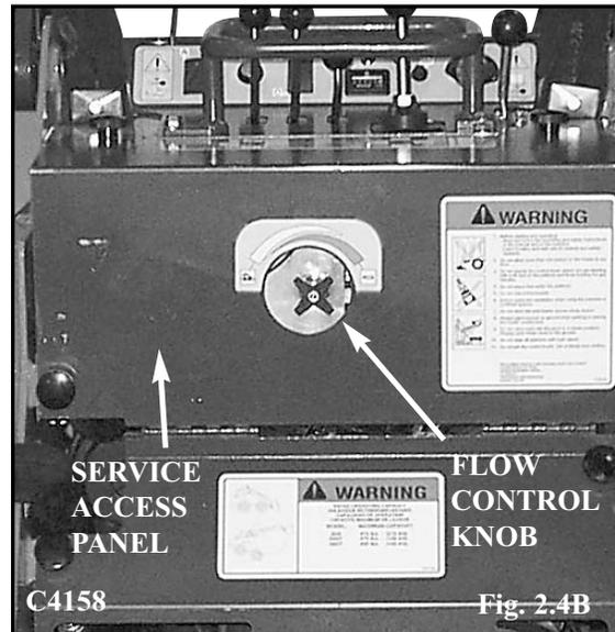
Turning the flow control knob clockwise will divert oil from the loaders drive system to the motor spool auxiliary circuit slowing the loaders travel speed. When fully turned in, approximately 1 gpm (3.8 l/m) of oil will still flow to the loaders drive system. This is the loaders slowest travel speed setting.
