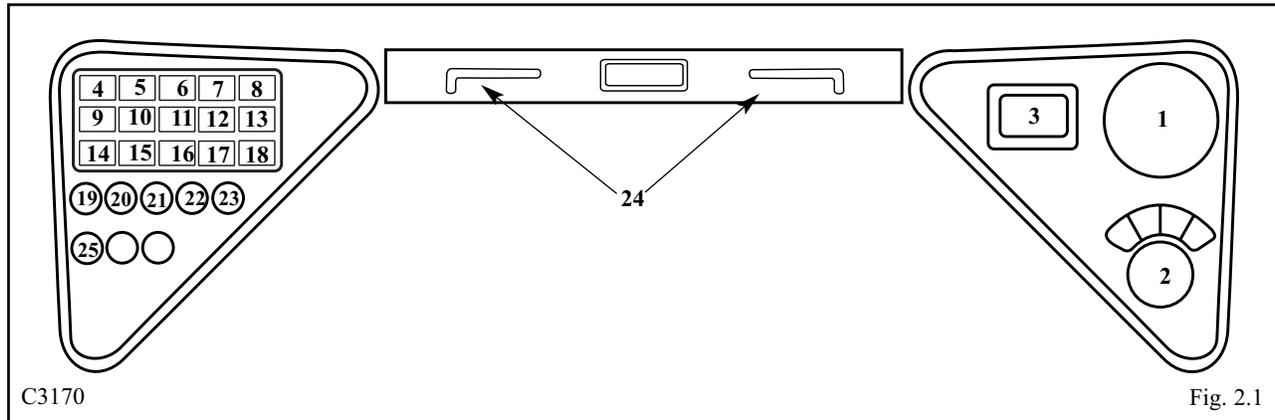
**1. Fuel Gauge:** The fuel gauge indicates the quantity of fuel remaining in the fuel tank.
