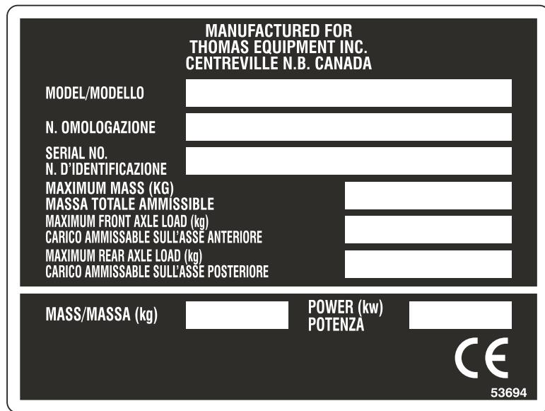
It is important when ordering replacement parts or making a service inquiry to provide both the model number and serial number of your Thomas loader. The serial number plate is located at the rear of the machine on the left hand side. In the event that the serial number plate is missing, the model number and serial number are both stamped into the main frame inside the rear door, right hand side, next to the fuel line shut off petcock. (fig. C4407)
