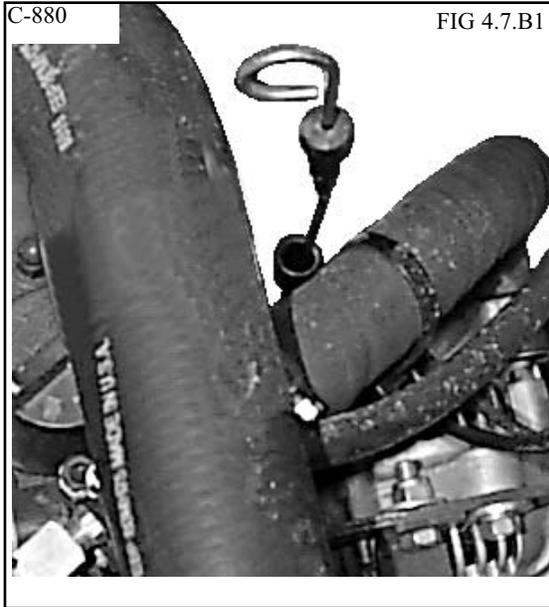
Keep the oil level between the full and low mark on the dipstick (Fig. 4. 7B2). Do not fill above the full mark and use only appropriate oil (See Section 5 for specifications).
