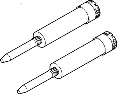
A line drawing of two identical adjusting pins. Each pin has a long, tapered shaft with a pointed tip, a threaded section near the base, and a cylindrical handle with a knurled end.                                        | ADJUSTING PIN FOR<br>CRANKSHAFT AND CAMSHAFT  | T243HDS  |
