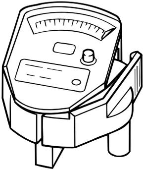
A line drawing of a toothed belt tension gauge. It features a semi-circular dial with a needle and scale, a central adjustment knob, and a handle with a finger loop. Two vertical pins extend from the bottom of the device. | TOOTHED BELT TENSION GAUGE<br><br>Quantity -1 | T243 HDS |
