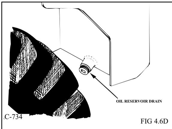
To drain the oil: remove the drain plug located at the bottom of the reservoir (Fig. 4.6D). Refill the hydraulic oil reservoir with engine oil See Section 5 for appropriate specifications).
