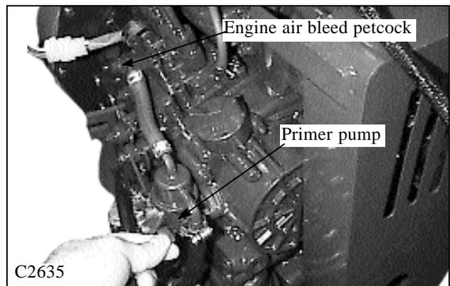
If the engine fails to continue operating, it may be necessary to bleed the fuel system of air after changing the fuel filter or running out of fuel. See Bleeding the Fuel System, next page.
