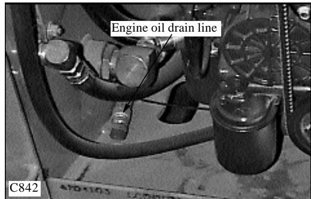
3 Place the line through the hole in the chassis and route to a container that will contain at least 8 liters (1.5gal) of fluid.
