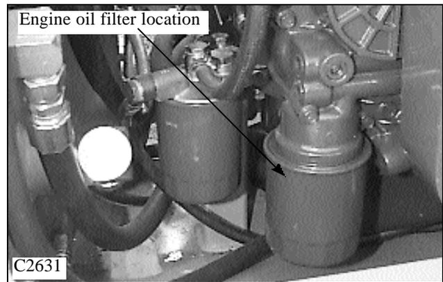
6 Check the oil filter mounting adapter area after removing the oil filter and check for dirt on the sealing surface and to make sure the oil filter O-ring seal has not stuck to the oil filter adapter.
