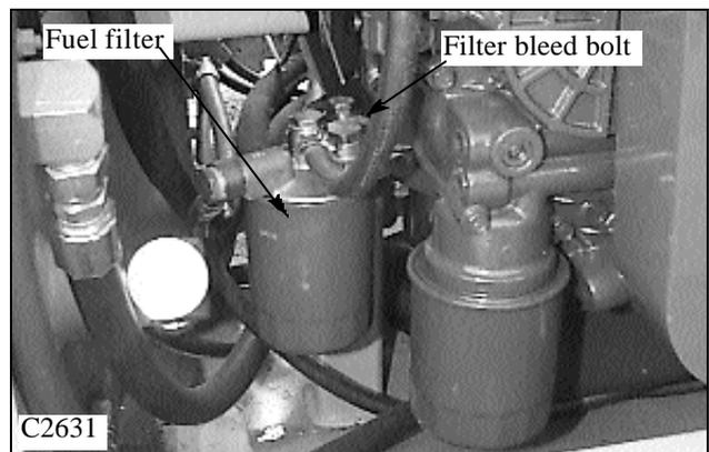
4 Lubricate the new fuel filter O-ring seal with light oil. Tighten the filter to the adapter mount hand tight.
