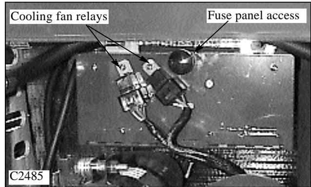
The relays are identical and may be checked by swapping one for the other to trace a malfunction. If changing the relays around does not repair the problem, the problem is either in the wiring, or in the actual electrical component.
