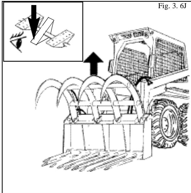
To close the grapple (Fig. 3. 6K), push down on the toe of the auxiliary pedal. The lift arm and the bucket pedals can be used to raise and tilt the grapple as with a bucket.
