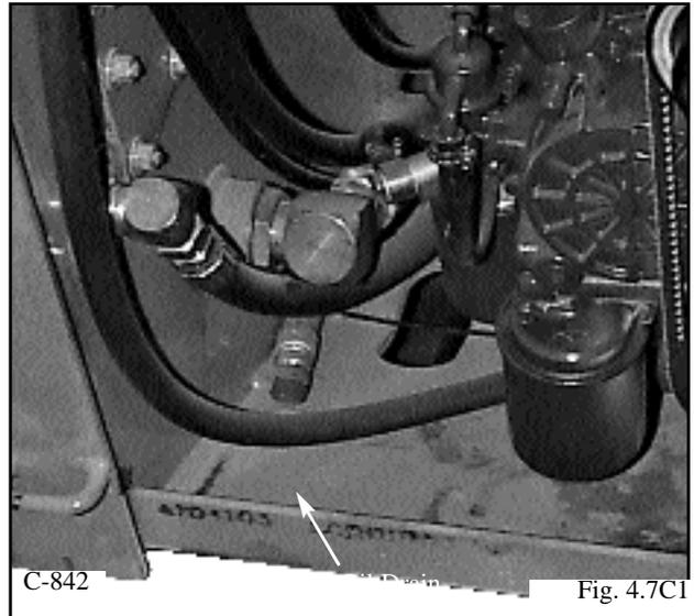
Remove the oil filter (Fig. 4. 7C2). Clean the filter housing surface. Put clean oil on the seal of the new filter and install the filter hand tight. Replace the oil drain plug. Remove the filler cap and add 10W30 API classification SE/CD engine oil. Start the engine and run for 5 minutes. Stop the engine and check for leaks at the filter. Recheck the oil level and add oil until the level is at the top mark on the dipstick.
