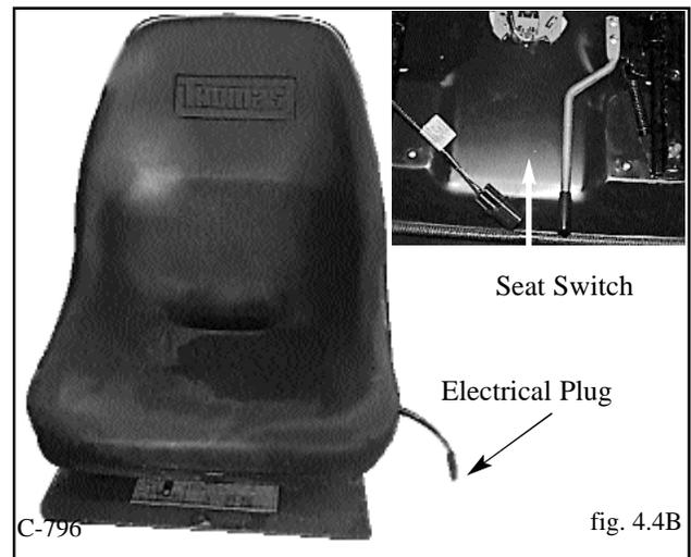
The seat and seat plate can be removed to provide access to the controls, hydraulic and hydrostatic components. To remove the seat assembly, remove the fasteners located at the front of the seat. **Disconnect the electrical plug!!** Lift the seat assembly out of the machine. When installing the seat, be sure the seat plate locks are in place at the rear (Fig. 4. 4B).
